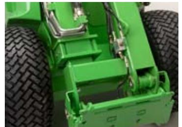
Hydraulic quick attachment coupling plate
