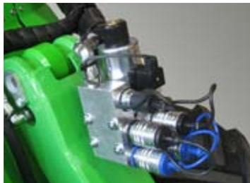
Two auxiliary hydraulics outlets in the front
